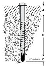
With the drill tool still in its hammer mode, drive the Crete-Flex® anchor using an appropriate hex or phillips drive tool until properly seated with the work surface. For installations using a rotary hammer drill, Elco offers two hex-shanked SDS masonry drill bits that can be used in conjunction with the 1000 installation tool: EMC120 for fasteners up to 2-1/4" in length, and EMC130 for lengths up to 4".
